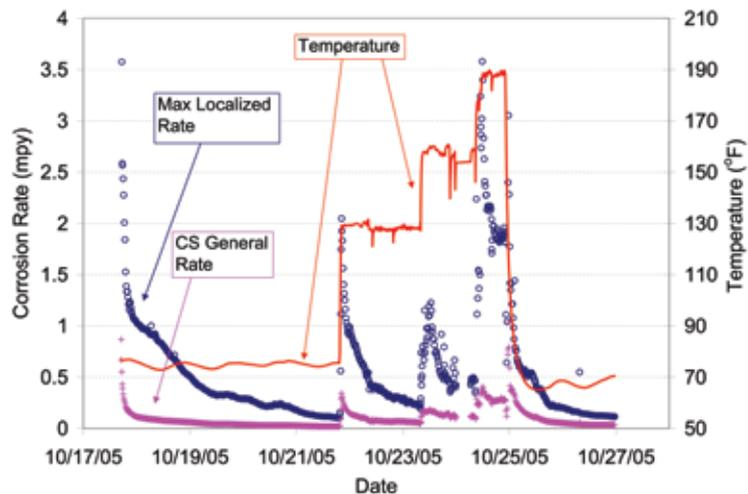
Localized and general corrosion rates of carbon steel 1008 in high-TDS/high-silica water.
