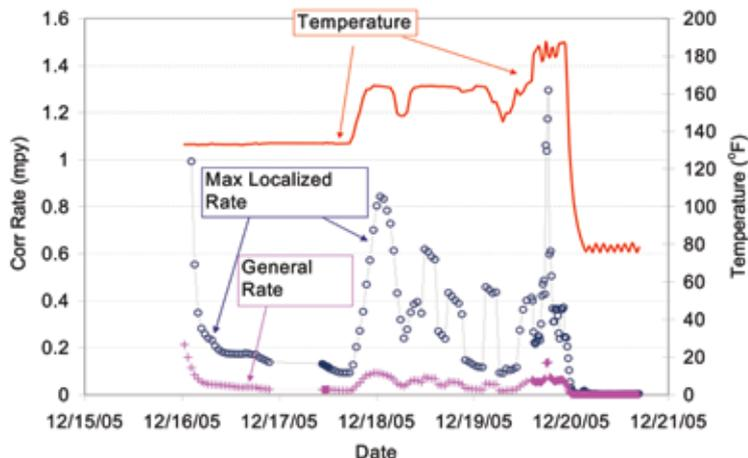
Localized and general corrosion rates of aluminum 1100 in high-silica/high-TDS water.
