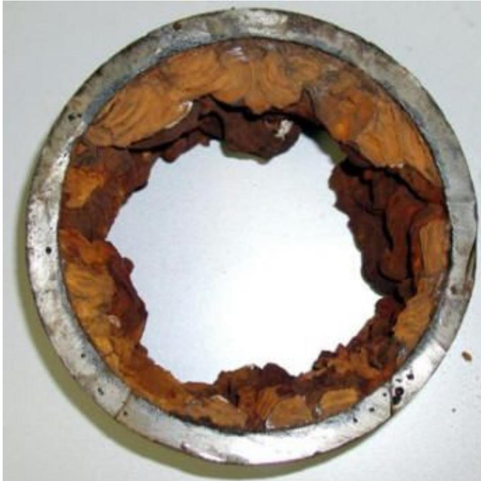
**Figure 1: Typical Constriction of Pipe due to Tubercle Buildup**
