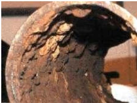
**Figure 2: Assorted Photographs of Tubercle formations due to Corrosion in iron/steel pipes**
